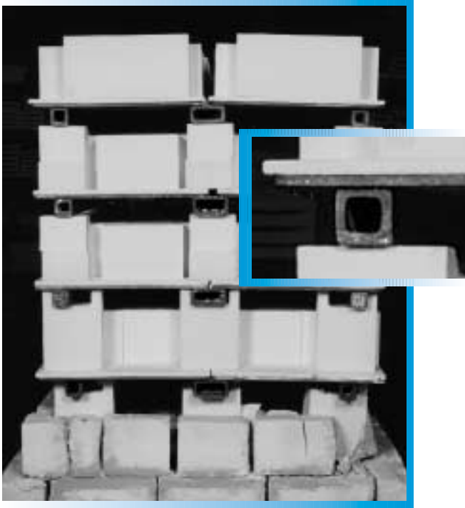
Before 4 Decks with Conventional 1-1/2" SiC Beams
